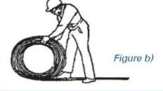
A short length of rope can also be rolled out over the ground as shown in Figure b).
