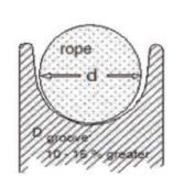
These measures will help ensure a very long service life which, at normal working loads, will be at least as long as that of wire ropes.
