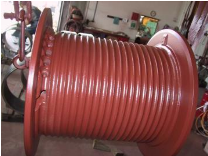
Drum winch with helical grooved barrel.
